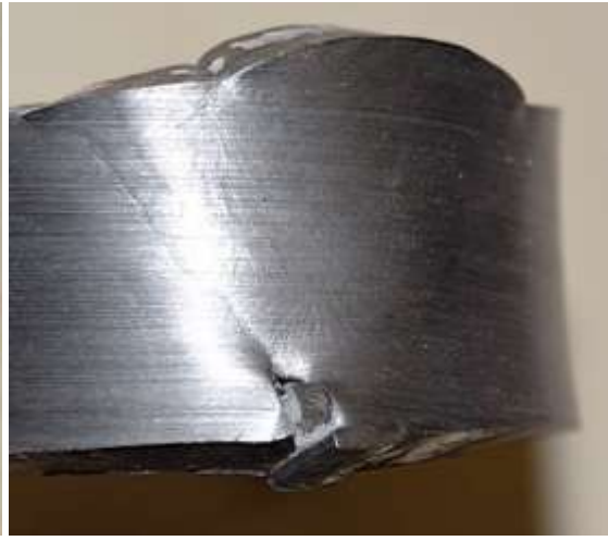
hibás varrat / wrong welded joint
